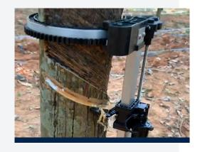
revolutionized the automation of extracting rubber from trees. Our microcontroller, micro-stepping motor controller and integrated low-dropout voltage regulator help provide more sustainable and resource-efficient agricultural production.
